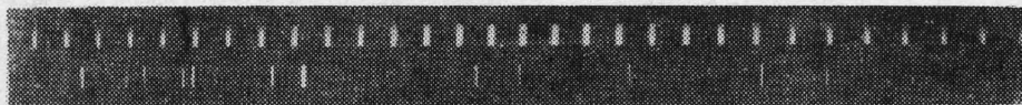
Fig. 4 Multi-order transmissive spectra from the F-P interferometer which consists of a pair of the coatings
