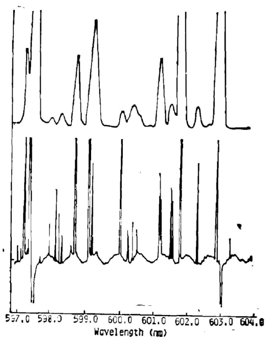
Fig. 3 Part of the optogalvanic signal of the Eu-Ne hollow cathode (lower trace) compared with the corresponding emission spectrum of the same hollow cathode lamp (upper trace)
