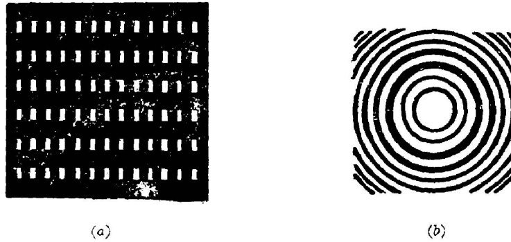
Fig. 3 Encoded grating combined by (a) Two directions and two spatial frequencies; (b) Both direction and spatial frequency changed continuously
