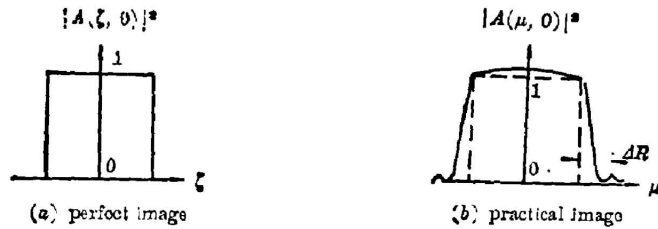
Fig. 6 Spread of reconstructed images caused by finite aperture of hologram (a) Ideal image; (b) Real image
