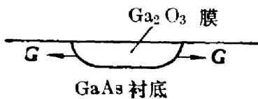
图4 条形氧化膜及应力示意图 Fig. 4 Schematic diagram of stripe-geometry oxide film and its stresses
