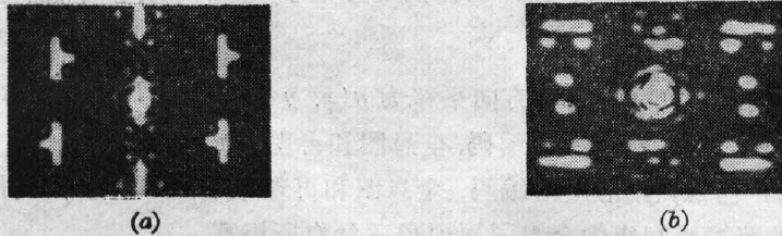
图6 (a) “上”和“-”相减产生的再现象; (b) “T”沿 y 方向微分产生的再现象 Fig. 6 (a) Reconstruction image of subtraction between Chinese character “上” and “-” (b) Reconstruction image of differentiation along y axis for letter “T”
