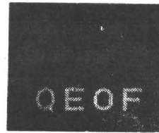
图 6 \mathbf{O}^1 的匹配滤波器只对 \mathbf{O}^1 有响应, 响应点也受到调制 Fig. 6 MSF of \mathbf{O}^1 is response to \mathbf{O}^1 only, the responding point is modulated too
