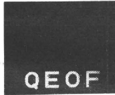
图 5 \mathbf{O} 的匹配滤波器对 \mathbf{Q} 也有响应 Fig. 5 MSF of \mathbf{O} is also response to \mathbf{Q}
