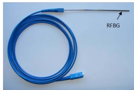
Fig. 10. Physical image of RFBG sensor encapsulated in alumina ceramic tube and Ni alloy shell [113] .
