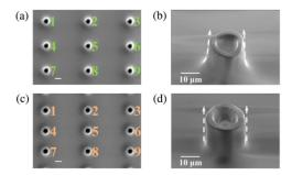
**Fig. 4.** SEM photos of microtube structures fabricated with high-order Bessel beams. (a), (b) Before and (c), (d) after aberration correction; the scaling bars without notation represent 20  $\mu$ m.
