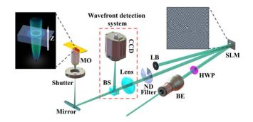
**Fig. 2.** Schematic of the setup. BE, beam expander; HWP, half-wave plate; SLM, spatial light modulator; LB, laser block; ND filter, neutral-density filter; BS, beam splitter; Shutter, mechanical shutter; MO, microscope objective; CCD, CCD camera. Inset close to the SLM presents the phase pattern to generate the Bessel vortex beams; the corresponding 3D light fields at the focus area in the slide are presented in the inset close to MO.
