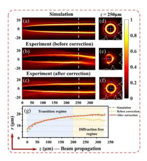
**Fig. 3.** Correction of the high-order Bessel beams with vortex charge m=6; the longitudinal intensity profiles along propagation (a) in simulation and in experiments (b) before and (c) after the correction; corresponding transverse intensity profiles at  $z=250~\mu m$  in (d)–(f); (g) evolution of the main lobe size along the propagation.
