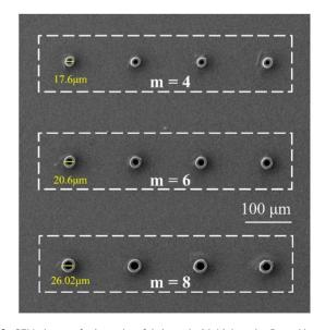
**Fig. 6.** SEM photos of microtubes fabricated with high-order Bessel beams of different vortex charges.
