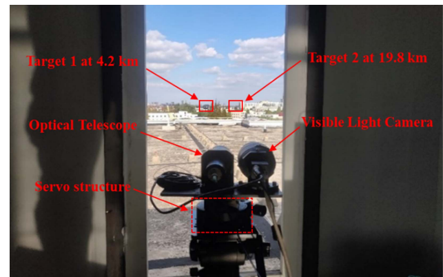
Fig. 7. Optical transceiver and target scenario in the field verification experiment.
