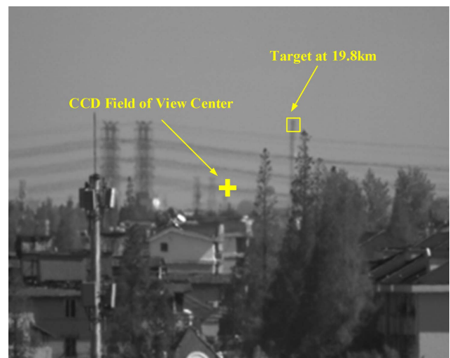
Fig. 10. Real target scenario at a distance of 19.8 km from the coherent lidar.
