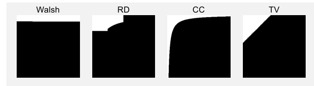
Fig. 2. Sampling diagrams in the Hadamard spectral domain for different sampling strategies [ p = q = 256 , SR = 10%].
