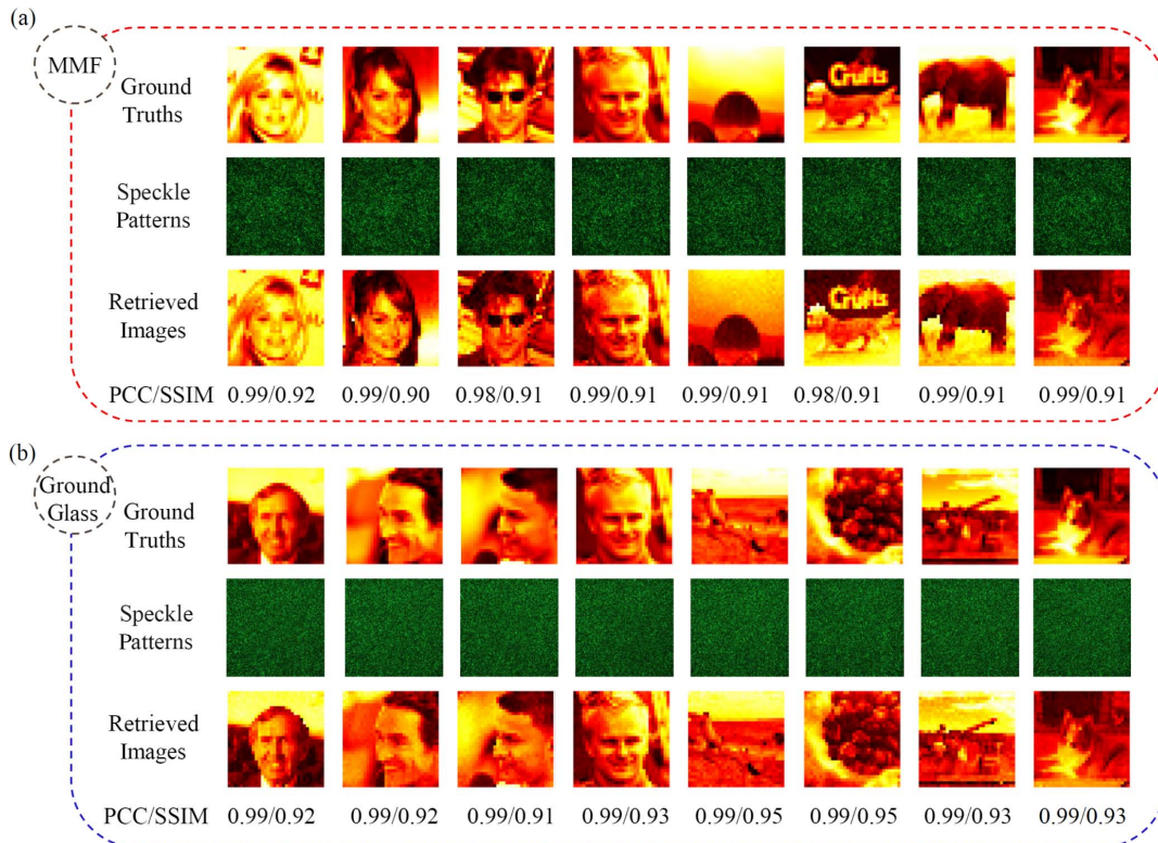
Fig. 4. Near-unity fidelity retrieval of 256-level grayscale phase-encoded images of human faces and natural scene images through (a) an MMF and (b) a ground glass, respectively. The ground truths, the corresponding distributions of the output speckle, and the retrieved images are provided. The resolution of all transmitted and retrieved images is 32 \times 32 . These images are adapted from the CelebA dataset [40] and the ImageNet dataset [41] , respectively.
