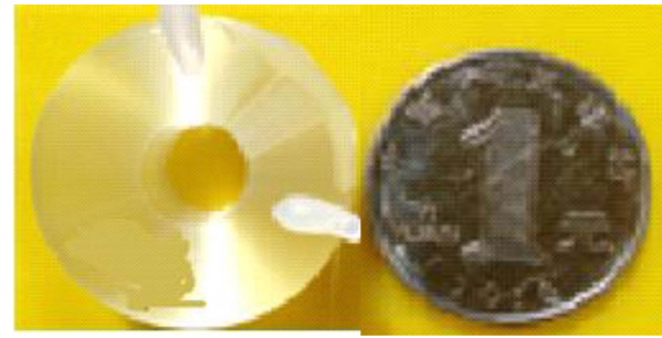
Fig. 3. Miniaturized optical fiber coil with coin for scale.
