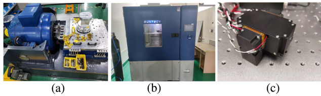
Fig. 9. Aerospace environmental tests equipment and the IF-ECDL for the tests. (a) Vibration test bench. (b) Temperature test chamber. (c) Developed IF-ECDL for the tests.
