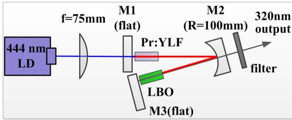
Fig. 1. Laser experimental setup.
