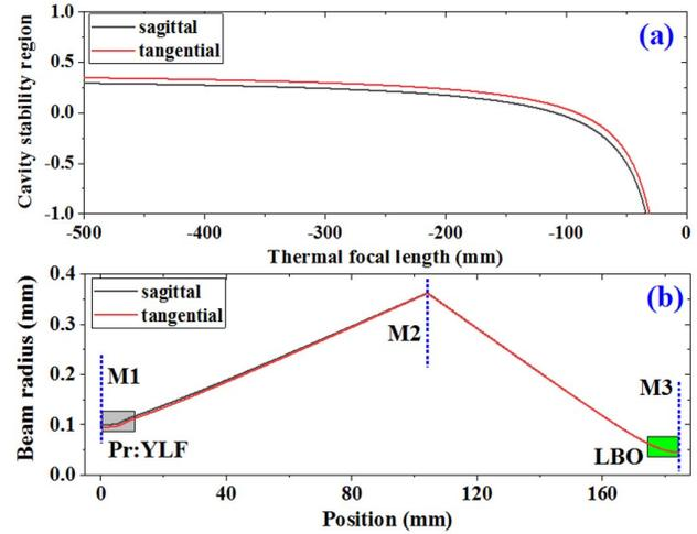
Fig. 2. (a) Cavity stability parameter versus thermal focal length of the laser gain medium; (b) beam sizes at different positions of the laser cavity.
