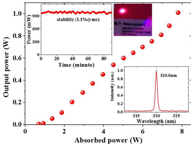
Fig. 4. Output power versus absorbed power of the 320 nm laser; inset: (top-left) output power stability and beam spot on a UV sensor card; (bottom-right) laser spectrum of the 320 laser.
