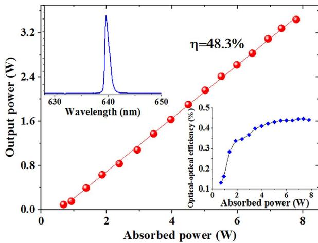
Fig. 3. Output power versus absorbed power of the 640 nm laser; inset: (top-left) laser spectrum and (bottom-right) optical-optical efficiencies.
