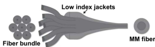
Fig. 21. Schematic diagram of a photonic lantern [151] .
