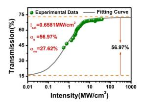
Fig. 1. Nonlinear optical transmission of CoOF-SA.
