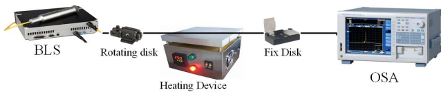
Fig. 4. Devices for torsion and temperature measurement.
