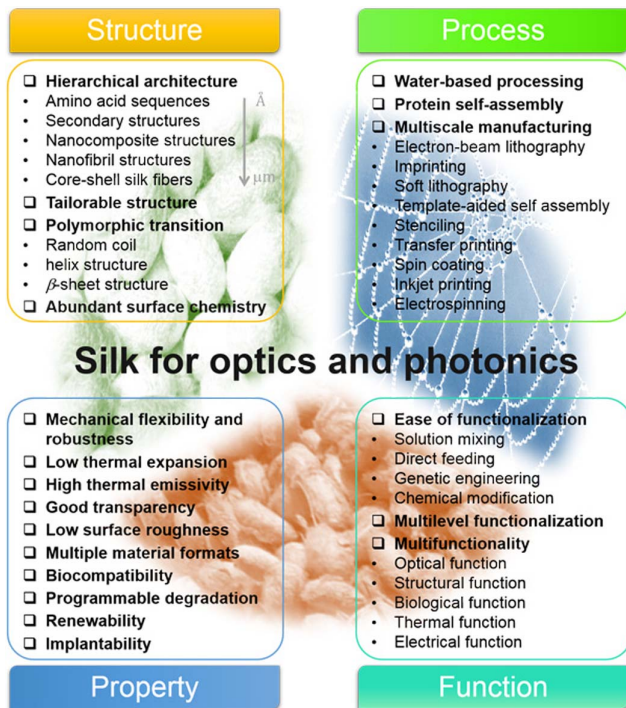
Fig. 2. Schematic representation of the inherent outstanding material characteristics of silk protein. The impressive balance of structure, process, property, and function makes silk distinct from other biopolymers.
