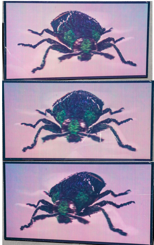
Fig. 7. Sample views of printed single-parallax digital hologram made of cloud of points. Final dimensions are 360 mm \times 190 mm.
