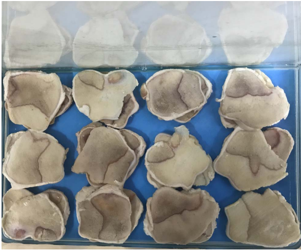
Fig. 2. Step of soaking swine slices into EDTA solution to imitate the process of bone loss.
