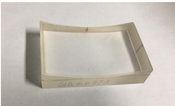
Fig. 5. Fabricated multi-curvature \alpha -quartz crystal on the glass substrate.
