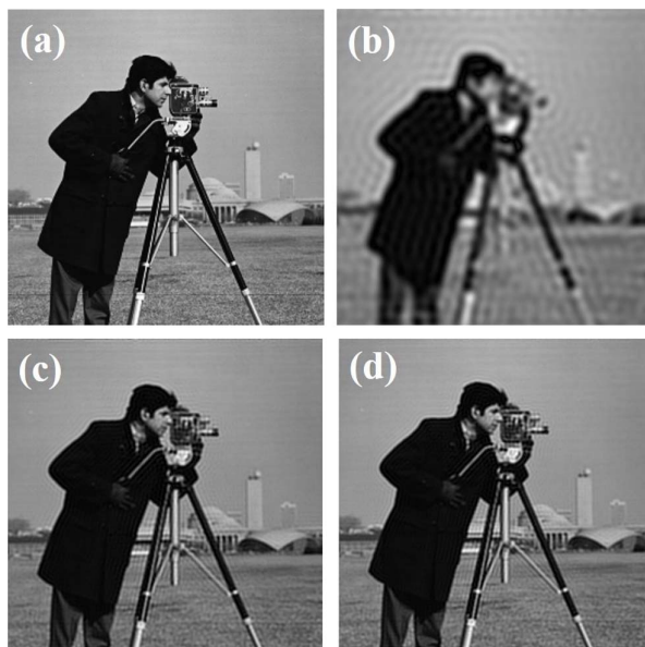
Fig. 3. The simulated imaging results restored by Tikhonov regularization. (a) Original image. (b) Restored image of individual subaperture. (c) Restored image of Ring6. (d) Restored image of effective aperture of Ring6.
