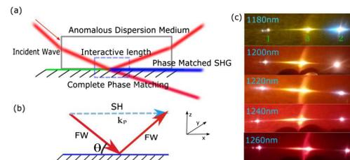
Fig. 1. (a) Diagrams of SHG generated by incident and reflected fundamental waves. (b) The triangle phase-matching type of the SHG spot. (c) The photographs of SHG with different fundamental wavelengths (1180 nm, 1200 nm, 1220 nm, 1240 nm, and 1260 nm).
