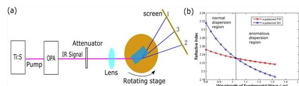
Fig. 2. (a) Experiment setup. (b) Comparison of the refractive index of an extraordinary-polarized second harmonic beam and that of an ordinary-polarized fundamental beam in a lithium niobate crystal.
