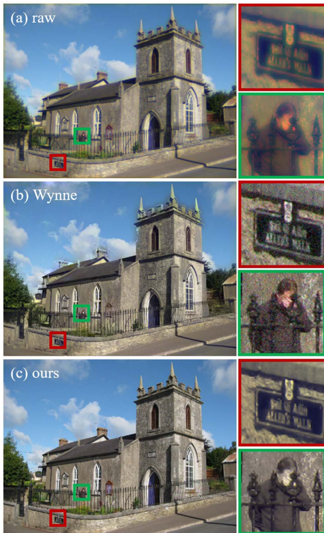
Fig. 7. Performance comparison of the conventional and our designs. (a) Raw image simulated with the proposed design. (b) Image simulated with Wynne's design. (c) Final corrected image with the proposed method. All of the results are simulated in Zemax with the image simulation function. Our joint design results outperform the conventional Wynne design.
