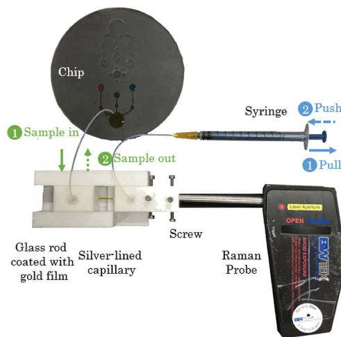
Fig. 2. Experimental diagram of the portable Raman probe extension kit.
