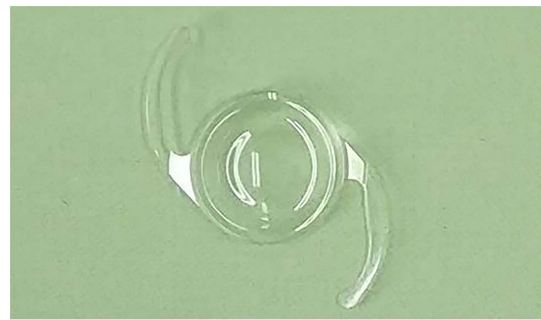
Fig. 7. Profile of the manufactured double-zone aspheric diffractive IOL.
