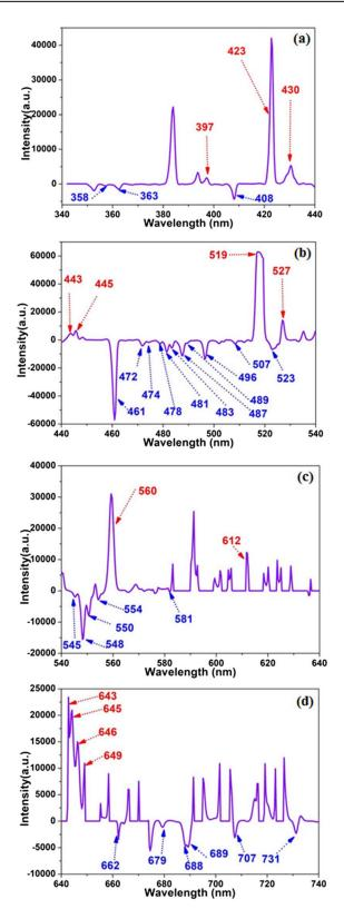
Fig. 4. (a) Intensities of 397, 423, 430 nm of Ca atoms and 358, 363, 408 nm of Sr atoms. (b) The intensities of 443, 445, 519, 527 nm of Ca atoms and 461, 474, 478, 481, 483, 487, 489, 496, 523 nm of Sr atoms. (c) The intensities of 560, 612 nm of Ca atoms and 545, 548, 550, 554, 581 nm of Sr atoms. (d) The intensities of 643, 645, 646, 649 nm of Ca atoms and 662, 679, 688, 689, 707, 731 nm of Sr atoms.
