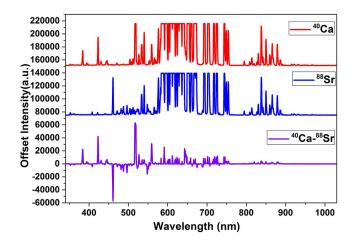
Fig. 3. Measured spectral intensities of Ca HCL (red line), Sr HCL (blue line), and the element-balance-detection signal with little effect of the buffer gas-lines (purple line).
