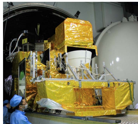
Fig. 12. Calibration system entering vacuum tank.
