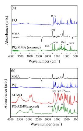
Fig. 5. Fourier transform infrared absorption spectra of PQ, monomers, and photoproducts.
