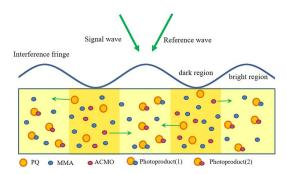
Fig. 7. Holographic diffusion process during exposure.
