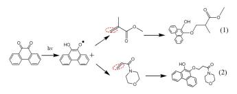
Fig. 6. Two kinds of different photoproducts (PQ attachment to the different monomer).
