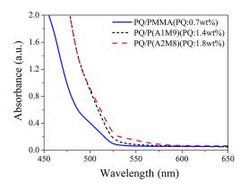
Fig. 2. Optical absorption spectra of different samples doped with different PQ concentration photopolymers.
