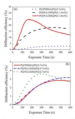
Fig. 4. Dependence of the orthogonal linear grating diffraction efficiency on the exposure time.
