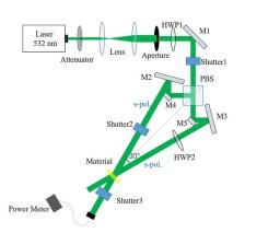
Fig. 3. Schematic of experimental setup. M: mirror; HWP: half-wave plate; PBS: polarizing beam splitter.
