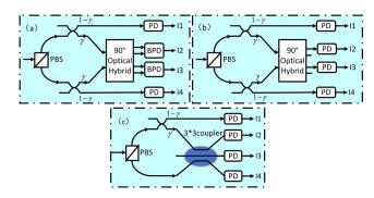
Fig. 2. Structures of SV-DD receivers. (a) Receiver A: with two BPDs, two PDs, and a 90° optical hybrid. (b) Receiver B: with four PDs, and a 90° optical hybrid. (c) Receiver C: with four PDs and a  $3 \times 3$  coupler.
