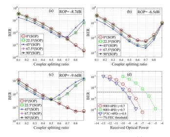
Fig. 6. Simulation results for the PDM-SC system: (a) BER vs. coupler splitting ratio for different SOPs for receiver A, (b) BER vs. coupler splitting ratio for different SOPs for receiver B, (c) BER vs. coupler splitting ratio for different SOPs for receiver C, and (d) BER vs. ROP for different SVRs in BTB transmissions.
