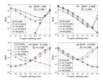
Fig. 7. Simulation results with 2.5 dB EL for the 90° hybrid and 0.15 dB EL for the  $3 \times 3$  coupler: BER vs. coupler splitting ratio for different SOPs (a) for receiver A for the PDM-IM system, (b) for receiver A for the PDM-SC system, (c) for receiver C for the PDM-IM system, and (d) for receiver C for the PDM-SC system.
