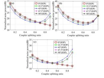
Fig. 4. Normalized noise power as a function of the coupler splitting ratio of the PDM-SC: (a) for receiver A, (b) for receiver B, and (c) for receiver C.
