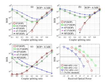
Fig. 5. Simulation results for the PDM-IM system: (a) BER vs. coupler splitting ratio for different SOPs for receiver A, (b) BER vs. coupler splitting ratio for different SOPs for receiver B, (c) BER vs. coupler splitting ratio for different SOPs for receiver C, and (d) BER vs. received optical power for different SVRs in BTB transmissions.
