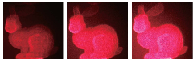
Fig. 13. Reconstructed real images using the proposed method. (left) The grayscale values of the bit planes B^0 , B^1 , and B^2 are 35, 65, and 110, respectively. (center) The grayscale values of the bit planes B^0 , B^1 , and B^2 are 60, 110, and 170, respectively. (right) The grayscale values of the bit planes B^0 , B^1 , and B^2 are 90, 150, and 255, respectively.
