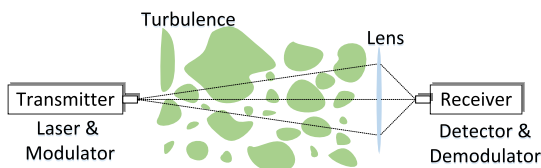
Fig. 1. Block diagram of an FSO system through the turbulent atmosphere.
