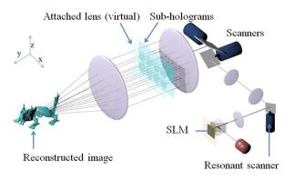
Fig. 3. Illustration of the CIH system integrated with a resonant scanner. Note that it is just an illustration and is not to scale.
