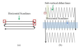
Fig. 2. Illustration of the sub-vertical scanning. (a) The galvanometer scan pattern, and (b) the dither scan pattern with the auxiliary scanner.
