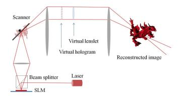
Fig. 1. Illustration of the CIH system.
