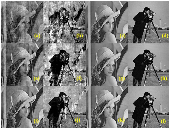
Fig. 6. Created complex field k_0(x, y) 1920 \times 1080 , reconstruction of the amplitude and phase at (a) and (b) 768 \times 768 , (e) and (f) 512 \times 512 , (i) and (j) 256 \times 256 by the conventional SCMM. Reconstruction of the amplitude and phase at (c) and (d) 768 \times 768 , (g) and (h) 512 \times 512 , (k) and (l) 256 \times 256 by the proposed method at 50 times iterations.
