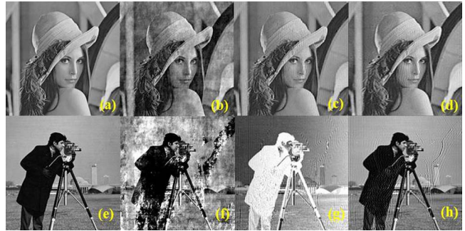
Fig. 5. Reconstructed amplitude and phase. (a) and (e) by the proposed method at 50 times iterations. (b) and (f) by the conventional SCMM. (c) and (g) by the off-axis method. (d) and (h) by the DPH method.
