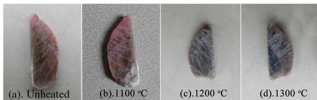
Fig. 1. Sample and its postheating color changes. (a) Photo of the unheated sample, photos of the sample heated at (b) 1100°C, (c) 1200°C, and (d) 1300°C.
