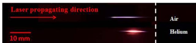
Fig. 2. Images of filaments in air and helium, which were captured by a digital camera (Nikon D7000: f number ( F ) = 5.6, light sensitivity (ISO) = 800, and shutter speed ( S ) = 1/13 s). The dashed line shows the position of the geometric focus. The arrows indicate the propagation direction of the femtosecond laser.
