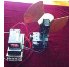
Fig. 4. Chopper wheel and its motor drive unit.
