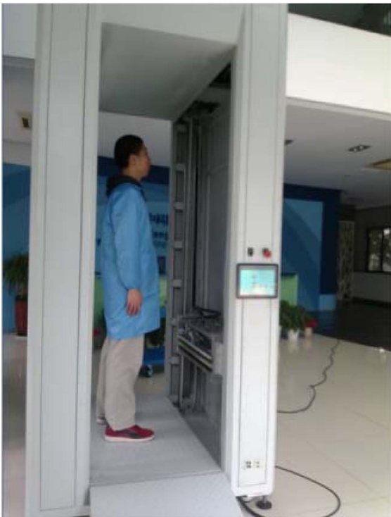
Fig. 2. Prototype of the wideband MMW imaging system.
