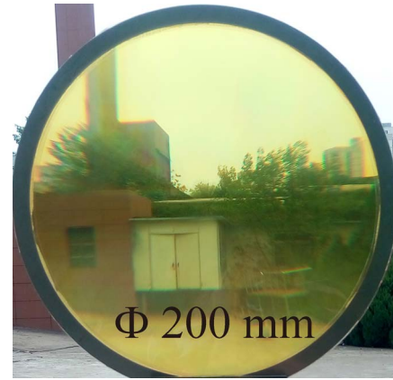
Fig. 7. A replicated four-level membrane FZL.
