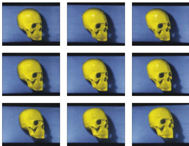
Fig. 10. Pictures taken from multiple directions of the holographic display digital 3D “skull.”
