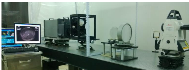
Fig. 7. Actual alignment process of channel 3 and the final interferogram.
