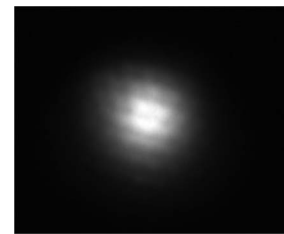
Fig. 3. Image of output beam of PPXRL at the distance of 30 cm from the CCD detector.
