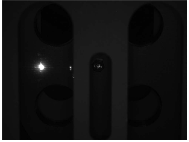
Fig. 7. Back-reflected light spot on the pinhole of the spatial filter.
