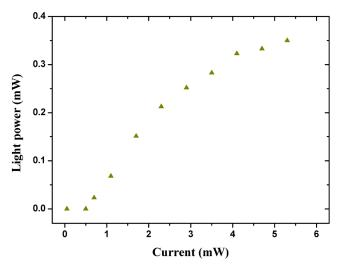
Fig. 4. L-I curve at ambient 25 °C.
