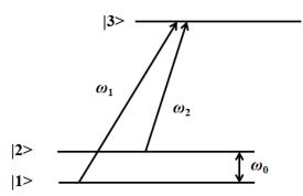
Fig. 1. Three level  $\Lambda$  system in alkali-metal atoms.
