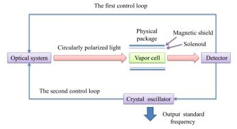
Fig. 2. Schematic view of a CPT atom clock.
