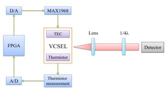
Fig. 3. Detailed setup of optical system.
