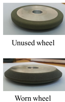
Fig. 8. Photos of grinding wheels before and after grinding.
