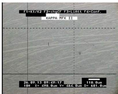
Fig. 9. Fomblin vacuum grease-coated optical sample surface.
