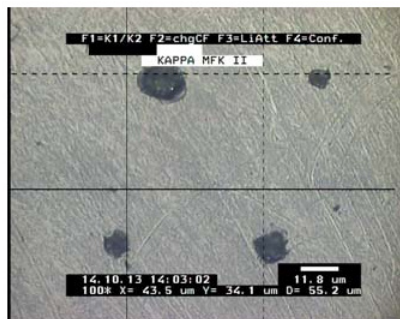
Fig. 10. UV radiation-induced damage of fused silica samples with vacuum grease contamination (one-on-one testing method).
