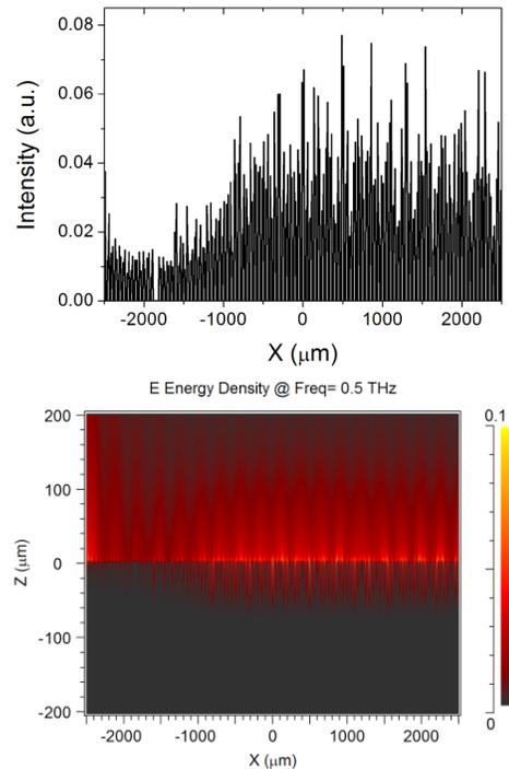
Fig. 4. (a) 1D and (b) 2D EM intensity ( $|E|^2$ ) distribution along the structured metal surface (grating 2) at a frequency of 0.5 THz.
