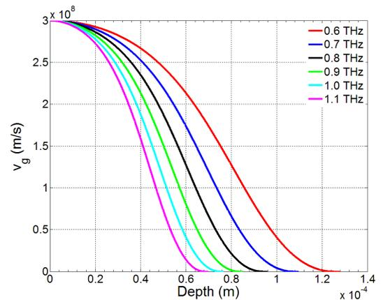
Fig. 2. Calculated group velocities ( $v_g$ ) of different grating depths ( $d$ ) at different frequencies: red line, 0.6 THz; blue line, 0.7 THz; black line, 0.8 THz; green line, 0.9 THz; cyan line, 1.0 THz; magenta line, 1.1 THz.
