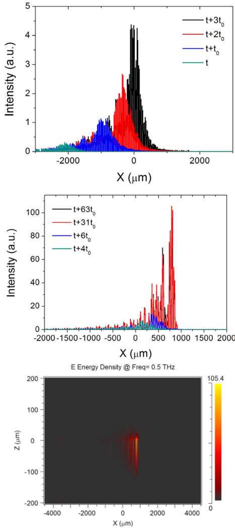
Fig. 3. Results of FDTD simulations. (a) 1D EM field distribution of grating 1 at different times and (b) 2D EM field distribution of grating 1 at the time of  $t + 63t_0$ . (c) 2D EM field distribution at the time of  $t + 63t_0$ .
