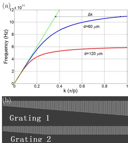
Fig. 1. (a) Dispersion curves calculated for different grating depths:  $d = 60 \mu\text{m}$  (blue line),  $d = 120 \mu\text{m}$  (red line), light in vacuum (green dotted line). (b) Schematic of a graded depth metal grating 1 and partial graded depth metal grating 2, with width ( $w$ ), period ( $p$ ), and depth ( $d$ ).
