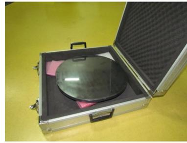
Fig. 12. Photo of the ground SiC mirror blank.
