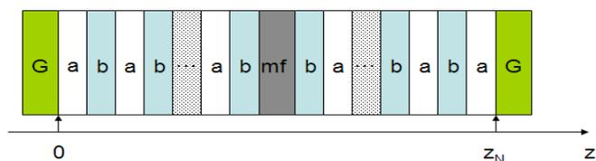
Fig. 1. The system structure of photonic crystals with a defect layer-filled with nanoparticle magnetic fluid.
