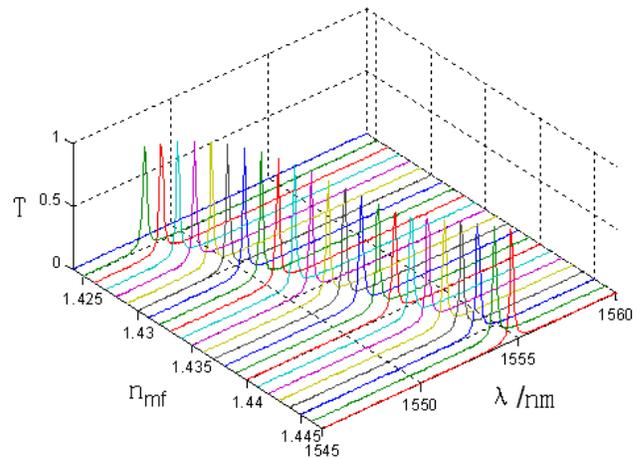
Fig. 2. The transmission spectra of photonic crystals at different refractive index  $n_{mf}$  of magnetic fluid.
