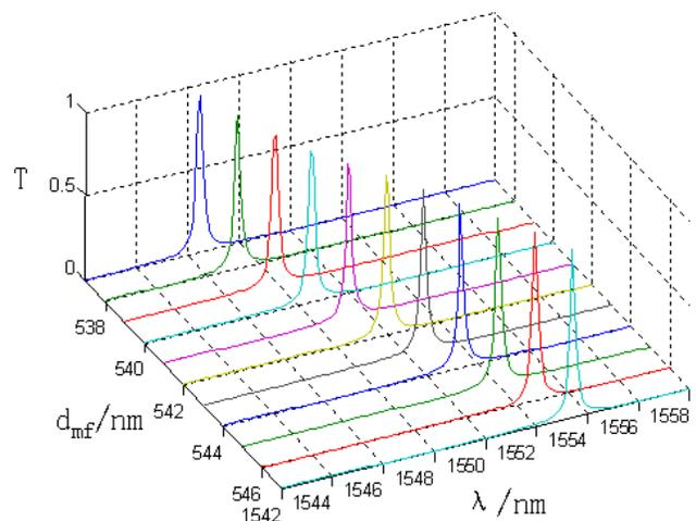
Fig. 3. The transmission spectra of photonic crystals as the change to thickness of the defect layer of magnetic fluid.
