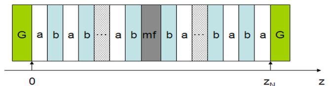
Fig. 1. The system structure of photonic crystals with a defect layer-filled with nanoparticle magnetic fluid.
